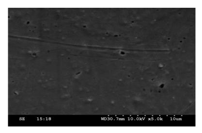
Figure 4: SEM of the film formed upto 220V in 0.1M L-ascorbic acid (glycolic medium) at room temperature (Magnification of the micrograph is X 5000)
