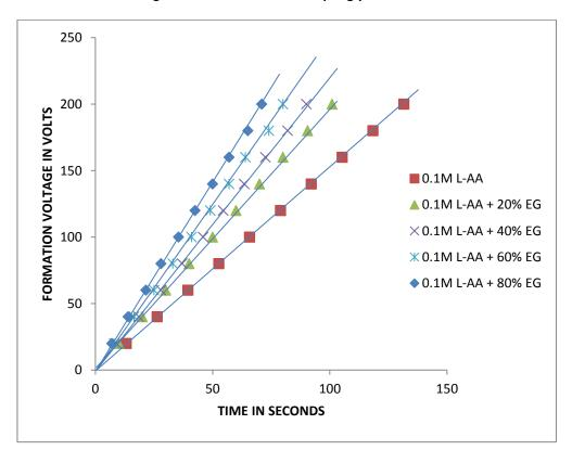
Table 1: Effect of solvent on the Anodization of Zircaloy-2 in 0.1 M L-Ascorbic acid
