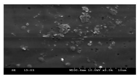
Figure 3: SEM of the film formed upto 220V in 0.1M L-ascorbic acid (aqueous medium) at room temperature (Magnification of the micrograph is X 5000)
